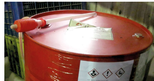
The labeling of containers with hazardous chemicals
