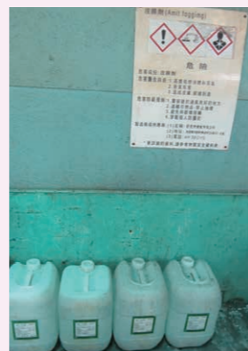
The labeling and posting of containers with hazardous chemicals
